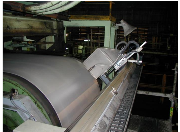
Detection of defects in metal coil surface
